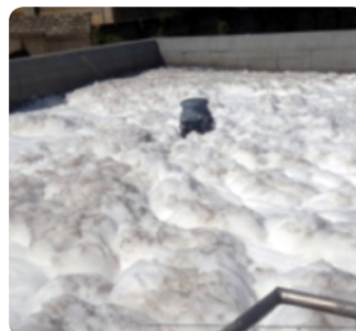
Waste water foaming before Chemical Leasing
